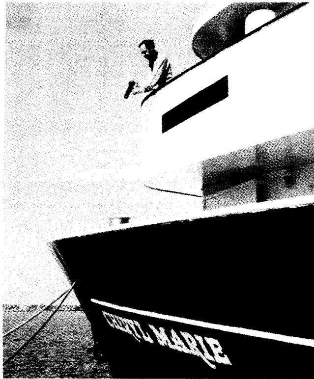
Figure 7.—Some fishing vessels are equipped with expendable bathythermograph systems. Temperature-sensing probes, released from a hand-held launcher, send data back to the vessel through fine conductor wires as they descend through the water.
