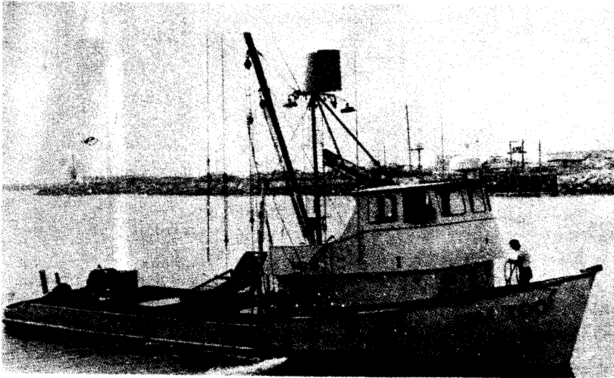
Figure 7.- Typical squid brailing vessel. Two lamps near the top of the mast are the attracting lamps.
