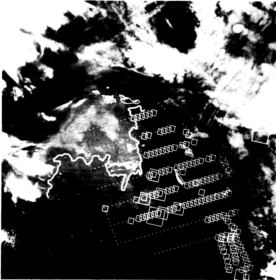
FIGURE 4. Distribution of anchovy eggs superimposed on the thermal image of the Southern California Bight taken 6 April, 1980. The 14^{\circ}\text{C} isotherm plotted from satellite gray-scale calibration has been drawn in. Feathery white objects are clouds. Squares indicate number of anchovy eggs under one square meter of sea surface.
