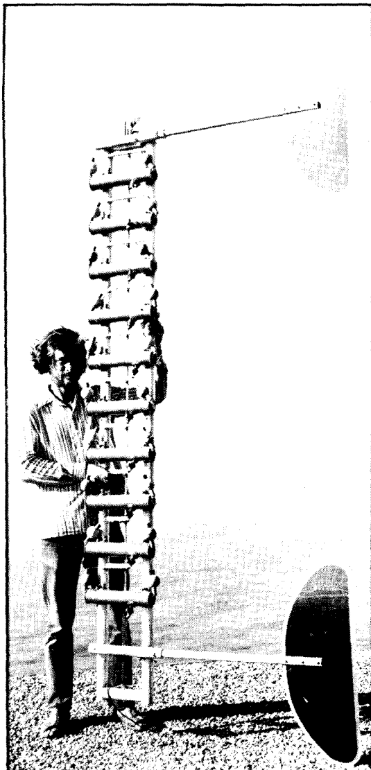
Figure 1. Micropatch sampler (MPS). The array is shown with ball valves open.
