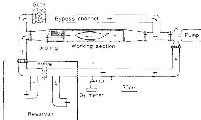
Fig. 1. Top view of albacore swimming respirometer. Arrows show direction of flow. Main return pipe is located at top of reservoir
