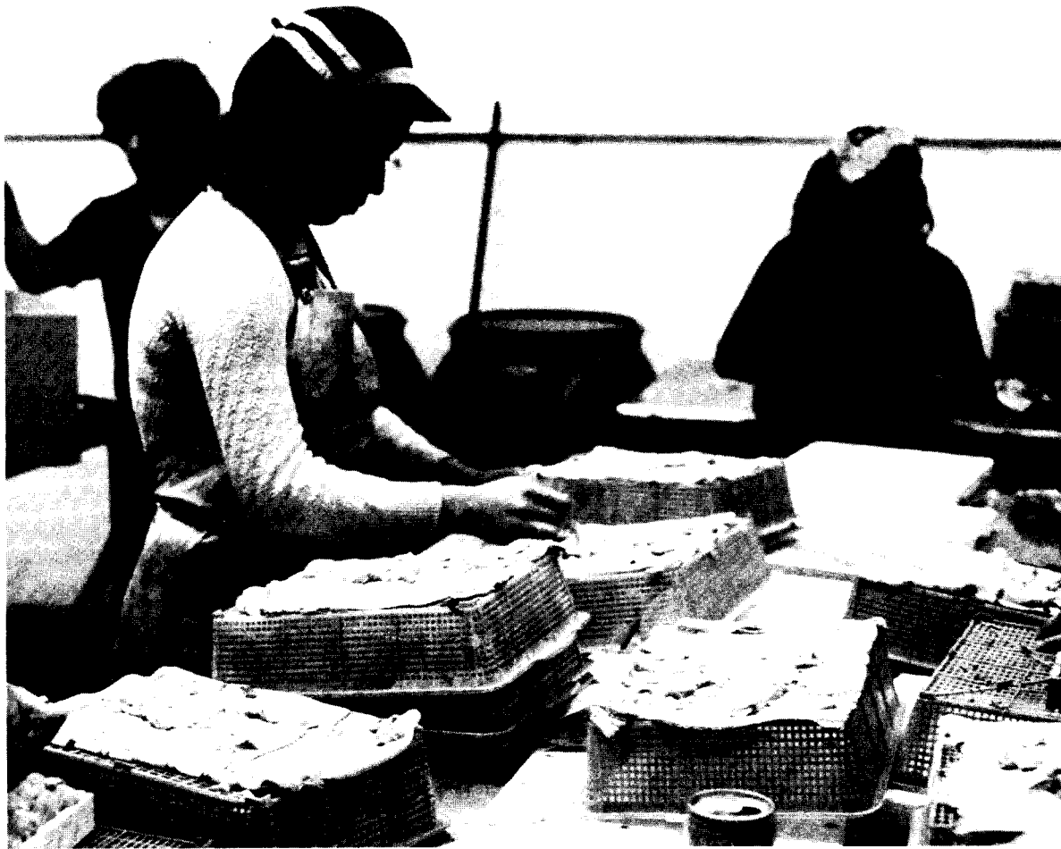
Figure 14.—Roe is drained thoroughly before packing; a layer of cloth helps absorb moisture.
