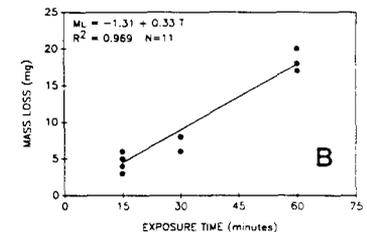
Figure 3.—Anode mass loss of corrosion timers and exposure time to seawater: A) in a laboratory experiment (salinity, 34.7‰; temperature, 23.5°C) and B) at the Hancock Seamount (salinity, 35.0‰; temperature, 15.5°C).
