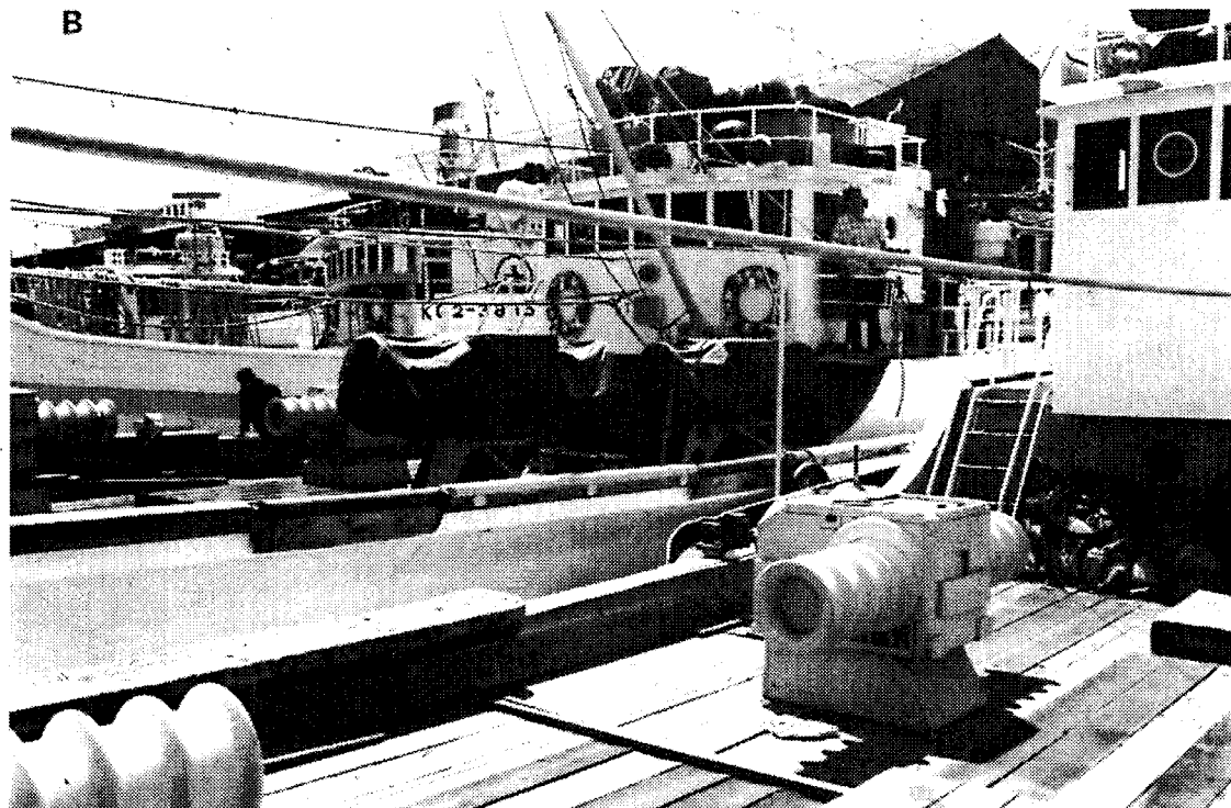
Figure 3.—B = Japanese coral fishing boat showing line haulers, tangle net dredges, and rollers on side of vessel.
