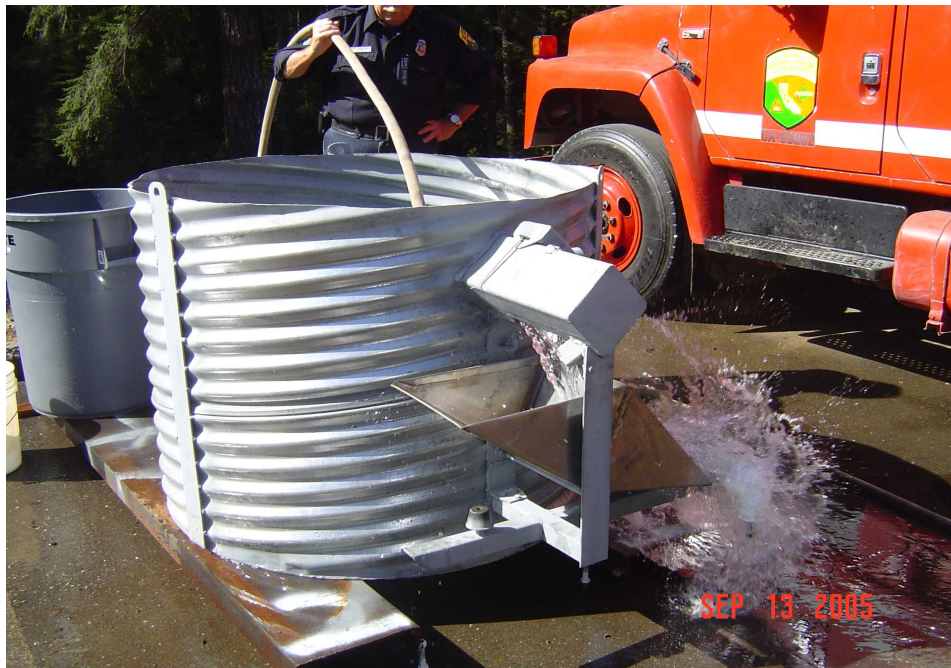
Fig. 1: The settling basin and tipping bucket during initial calibration. The settling basin, made of 122 cm (48”) diameter corrugated metal pipe, catches runoff from the road segment, allowing coarse sediment to settle. The runoff then passes through a rectangular arm and into the tipping bucket, shown here just after having tipped to the right. A subsample intake opening, obscured by the water in this photo, catches a 5-ml flow sample, which is routed to a bucket from which a composite sample is later collected for laboratory analysis of suspended solids.
