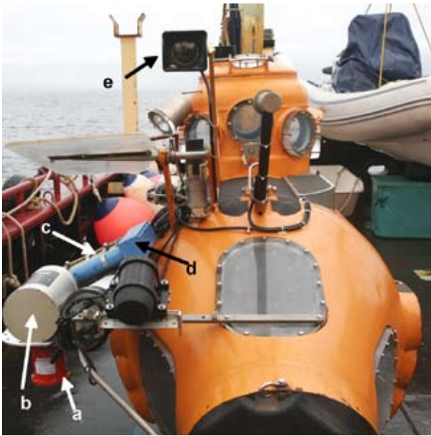
Figure 2. Sensors mounted to the Delta submersible: (a) Doppler velocity logger; (b) ring laser gyro; (c) color video survey camera; (d) paired scaling lasers; and (e) low-light video camera.
