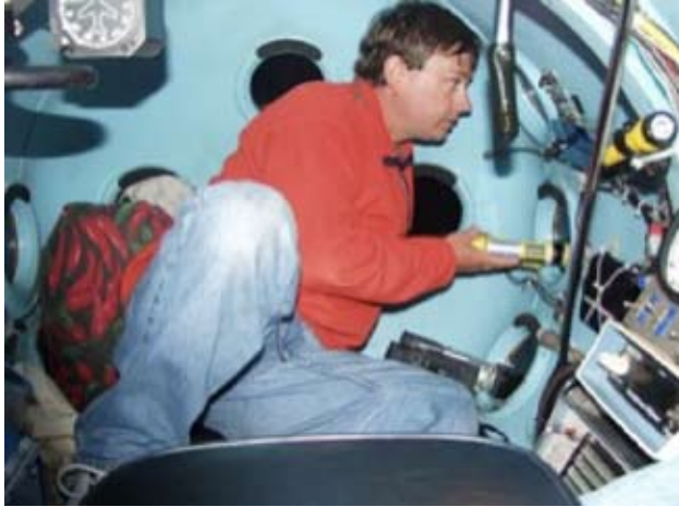
Figure 3. Scientific observer estimates distance to an underwater target by using a handheld sonar gun from inside the Delta submersible.
