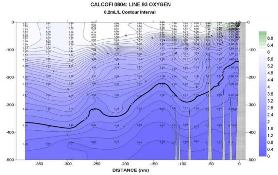
**Figure 8.** Oxygen values (ml/l) generated during the last CalCOFI cruise (24 March- 9 April) revealed low dissolved oxygen levels, particularly along the southern lines.
