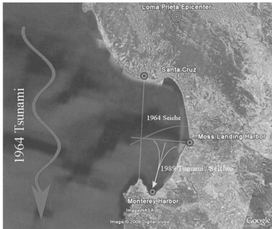
Figure 1. This figure shows Monterey Bay and depictions of the 1964 Great Alaskan Earthquake (GAE) tsunami (outside the bay) and the corresponding seiche (inside the bay), and the 1989 Loma Prieta Earthquake (LPE) tsunami and seiche (both inside the bay). The dotted line across the entrance of the bay represents the assumed location of the nodal line that corresponds to the node for transverse oscillations whose orientation is orthogonal to this line.
