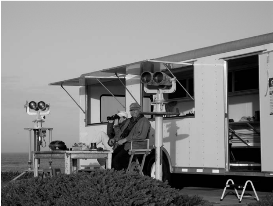
Figure 2. Observer station including mounted 25X binoculars for search to the horizon offshore and hand-held binoculars for tracking animals near shore.
