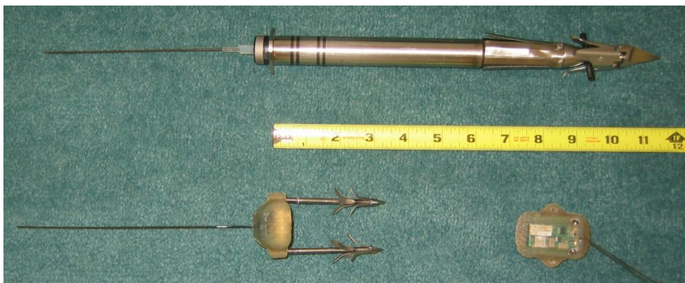
Fig 1. - Examples of a body-penetrating (Type I, ONR, 2009) (top) and a dorsal fin-penetrating (LIMPET, Type II, ONR, 2009) satellite transmitters.
