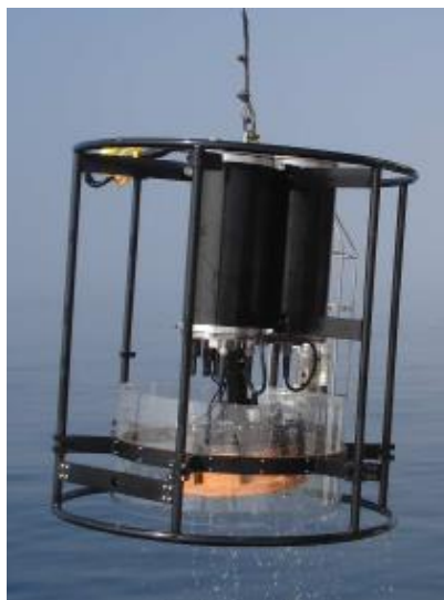
Figure 1.11. Cast echosounder systems are used to position echosounders and deep-water transducers closer to demersal fish targets. In this case, the transducer is gimballed to provide vertical measurements, irrespective of platform tilt due to, e.g. water current.
