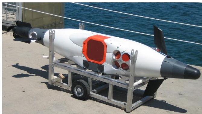
Figure 1.12. An autonomous underwater vehicle (AUV) fitted with a split-beam echosounder and an acoustic Doppler current profiler.
