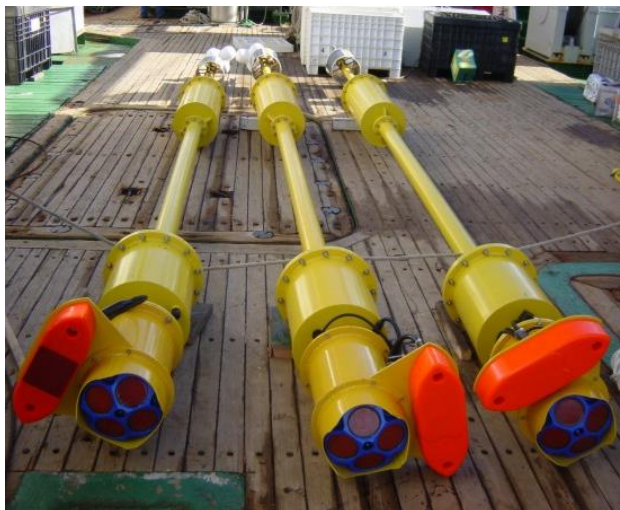
Figure 1.13. Buoys fitted with dual-frequency and split-beam echosounders, and acoustic Doppler current profilers.
