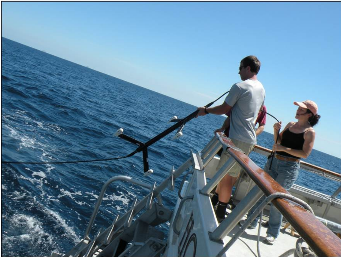
Figure 6.--Acousticians handling the volumetric array prototypes, torpedo array (top) and X-array (bottom), during a sea trial.
