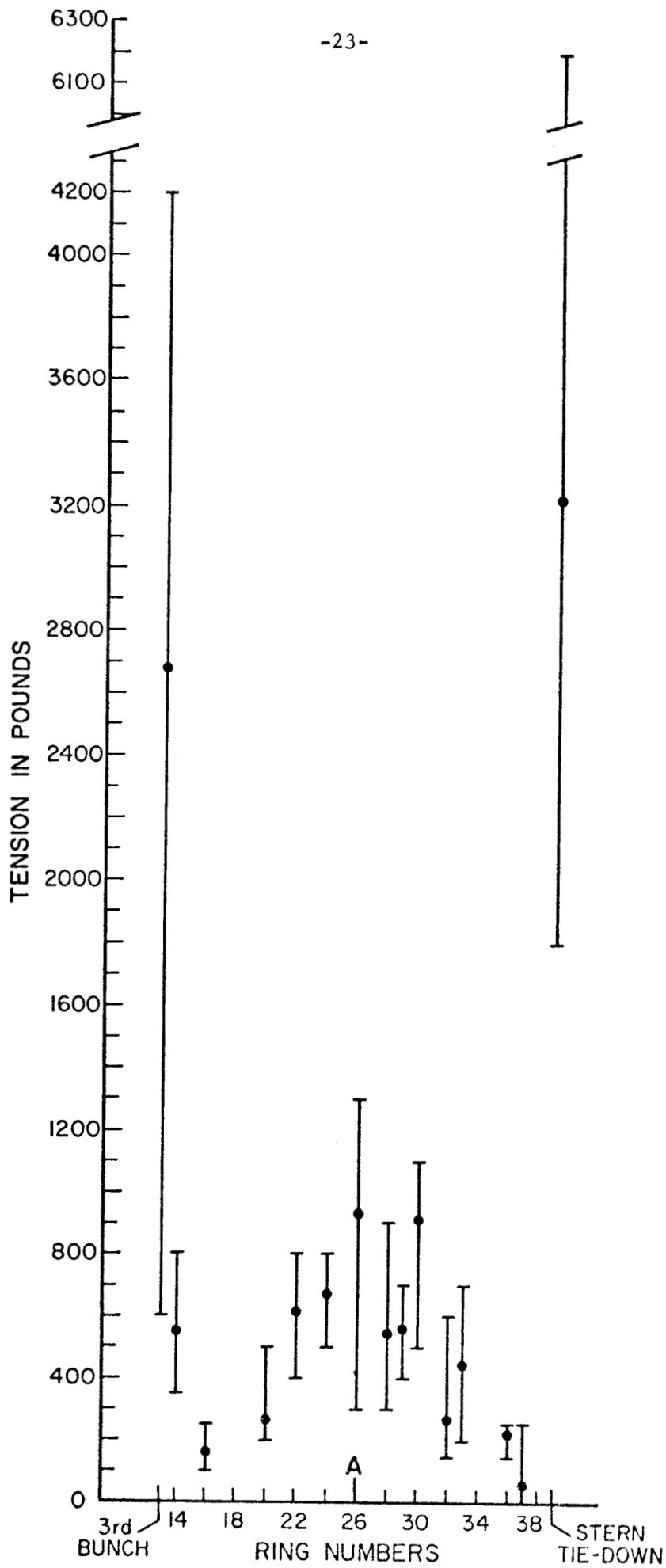
Figure 6. Distribution of tensions during backdown.
