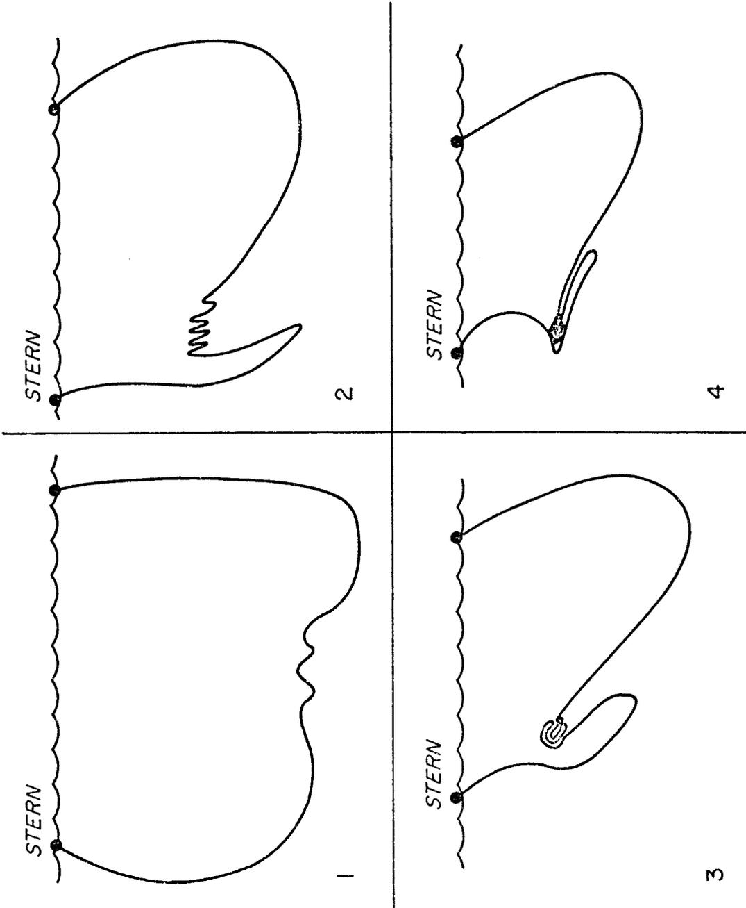
Figure 7. Backdown channel cross section during backdown showing development of stern sway.
