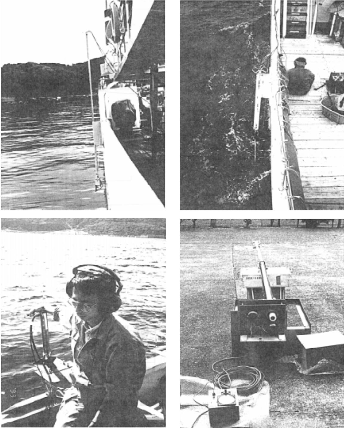
**Figure 4.** Hydrophone and pole rotating system.
