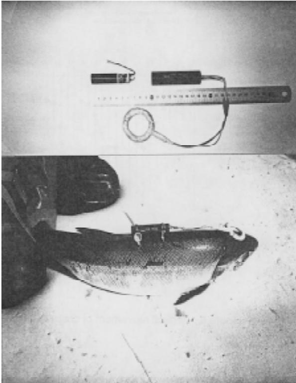
**Figure 8.** Artificial magnetic field generator attached to a chum salmon.
