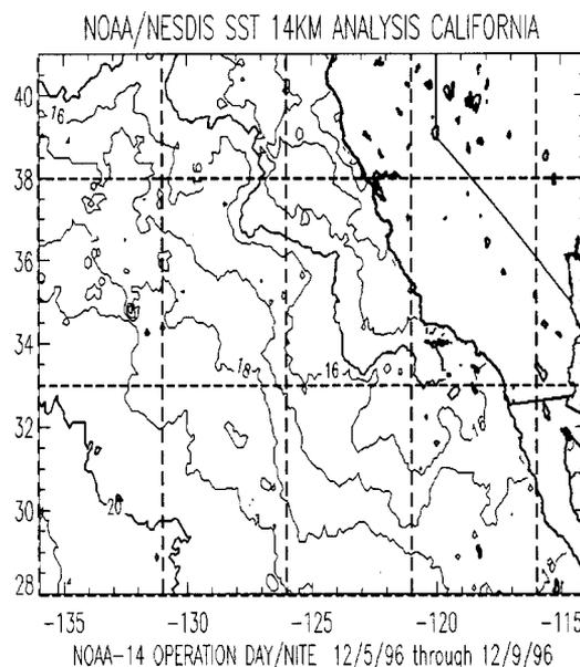
**Figure 1.** 14 km SST isotherm contour chart. Sample operational 14 km SST isotherm contour chart produced from objective analysis of 8 km observations of SST derived from AVHRR/2 visible and infrared data. These charts are generated twice a week using all satellite observations obtained since the previous chart production.
