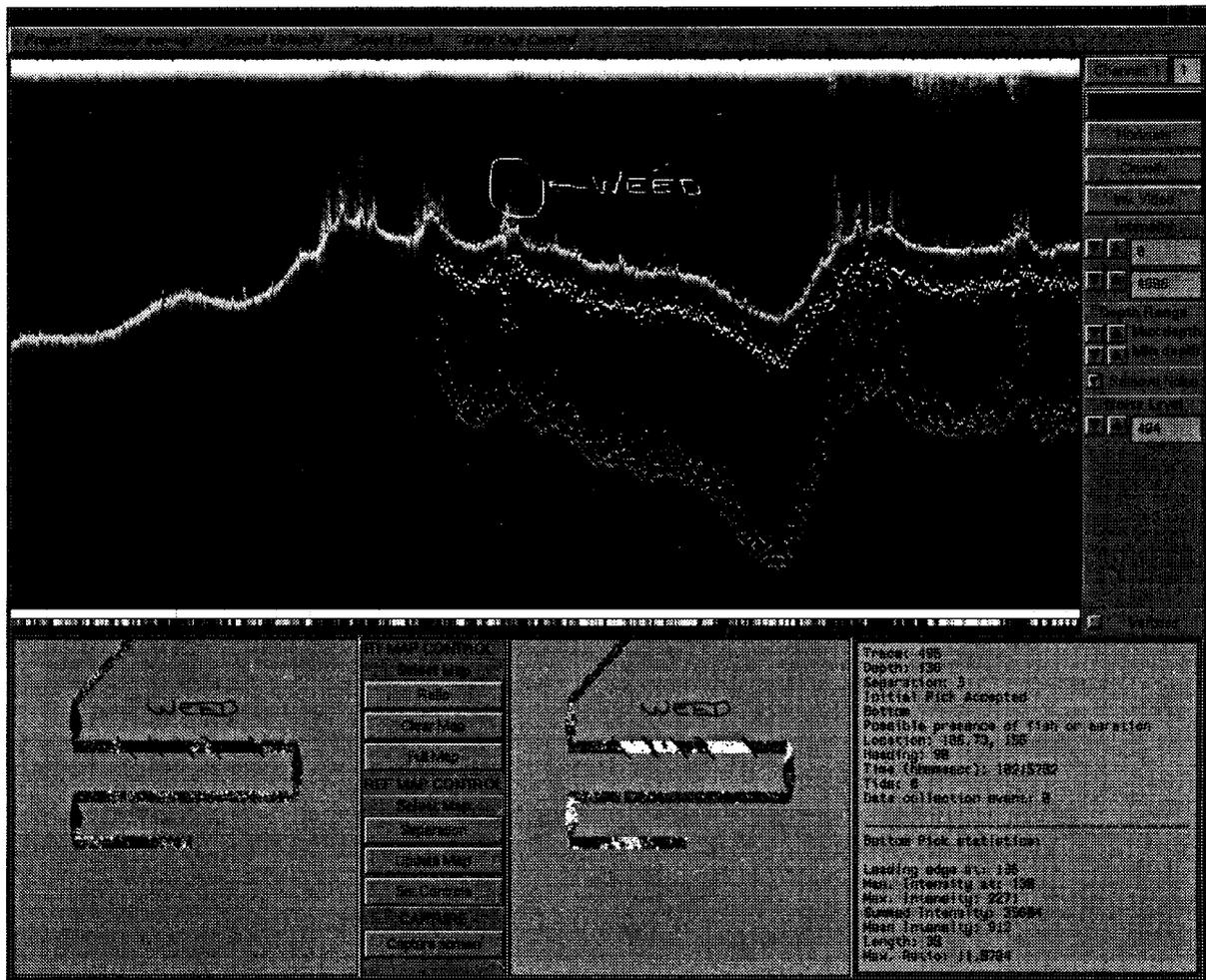
**Figure 6.** Example of TraceEd tool. Multiple horizons are traced as acoustic returns come in and various parameters used to distinguish characteristic features. Here the separation between bottom pick and earlier arrivals is used to identify seaweed. Distribution is simultaneously plotted in geographic space
