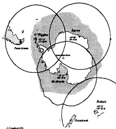
**Figure 3.** The nominal reception limit of NASA's McMurdo station is shown for three international SAR satellites. The other 3 ground stations are operated by Germany (O'Higgins), Japan (Syowa), and Australia (Hobart).
