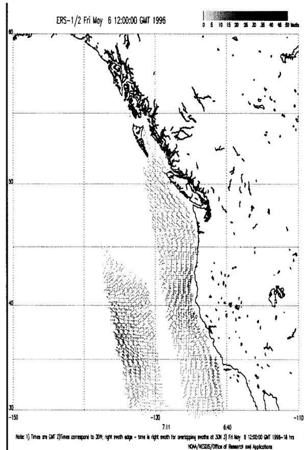
**Figure 4.** ERS-1 wind chart. Wind barb display of ERS-1 winds generated by the European Space Agency from the AMI Wind Scatterometer for an 18 hour period on May 6, 1996. Experimental charts like this for any region of the world are available on-line from the NOAA/NESDIS Office of Research and Applications (Chang 1996).
