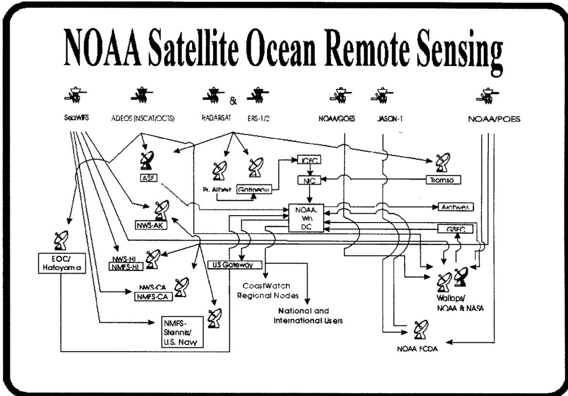
**Figure 6.** NOAA ocean satellite data reception and distribution. High-level schematic drawing of NOAA satellite reception facilities, data links, processing facilities, and distribution/archival network.
