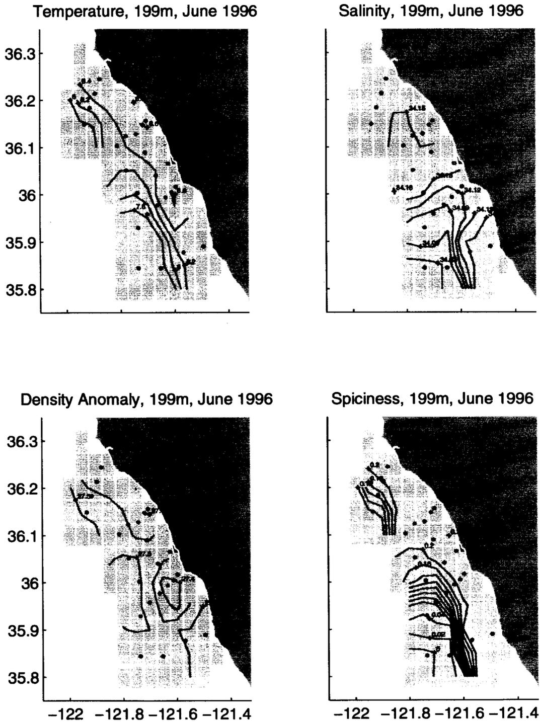
Figure 11. (a) Temperature, (b) salinity, (c) density anomaly, and (d) spiciness<sup>1</sup> measured at 199 m depth. Otherwise, same as Figure 9.
