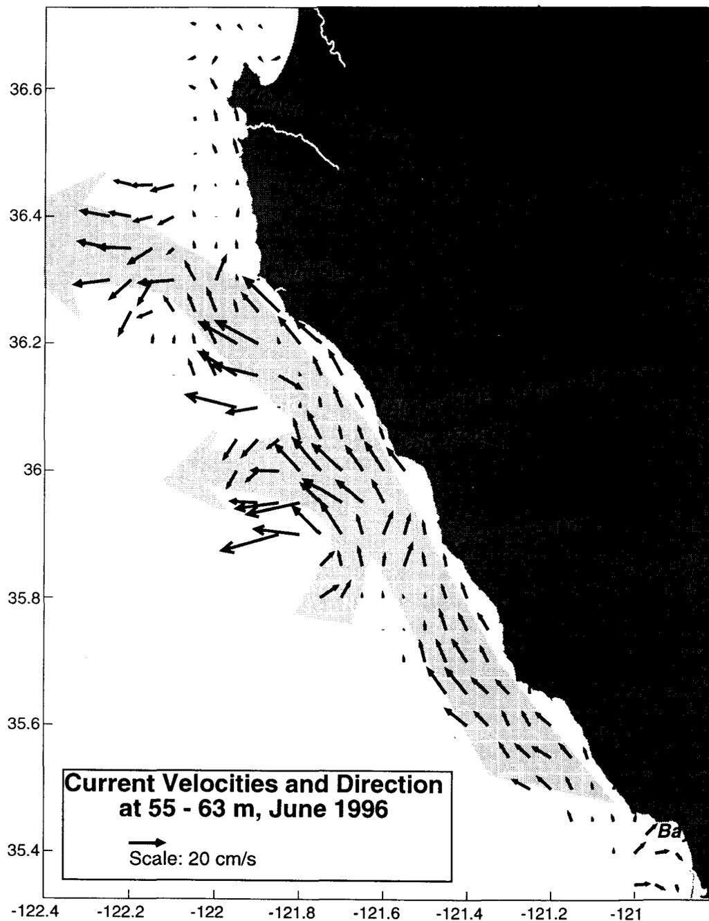
Figure 18. Conceptual model (large gray arrows) of ocean circulation off the Big Sur coast, as derived from current velocity and direction (small black arrows) measured with ADCP on the NOAA ship *McArthur*, 3-6 June 1996.
