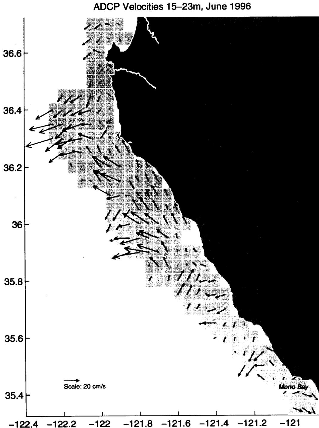
Figure 7a. Horizontal maps of ocean currents (ADCP velocity vectors) from Monterey to Morro Bays, 2-6 June 1996, averaged over 15-23 m water depth. Velocities over a (0.1 x 0.1)-degree region were gridded into 0.05-degree bins. Bins containing data are filled with light gray. The approximate region of the Big Creek Ecological Reserve is indicated with darker fill.
