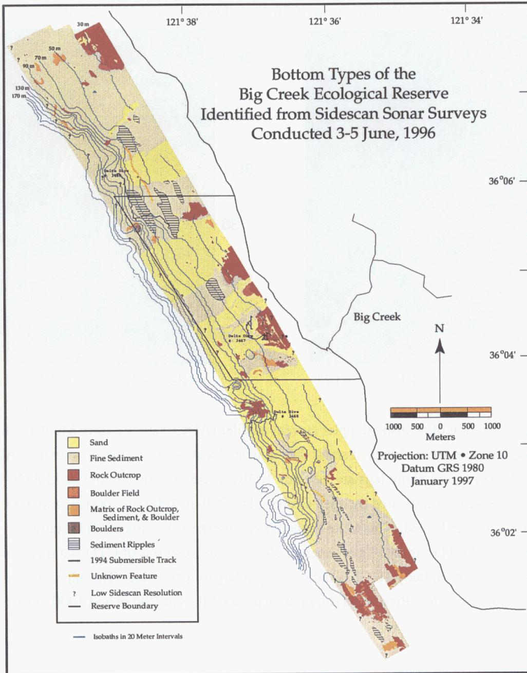
Figure 3a. Map of bottom types of the greater Big Creek Ecological Reserve (boundary indicated) area, as interpreted from a side scan sonar survey conducted 3-5 June 1996. Track lines from three submersible dives conducted in 1994 also are indicated. Question marks indicate areas of low resolution of the acoustic signal (see text). Isobaths are in 20-meter intervals. Table 3 includes estimated sizes of individual boulders and pinnacles.
