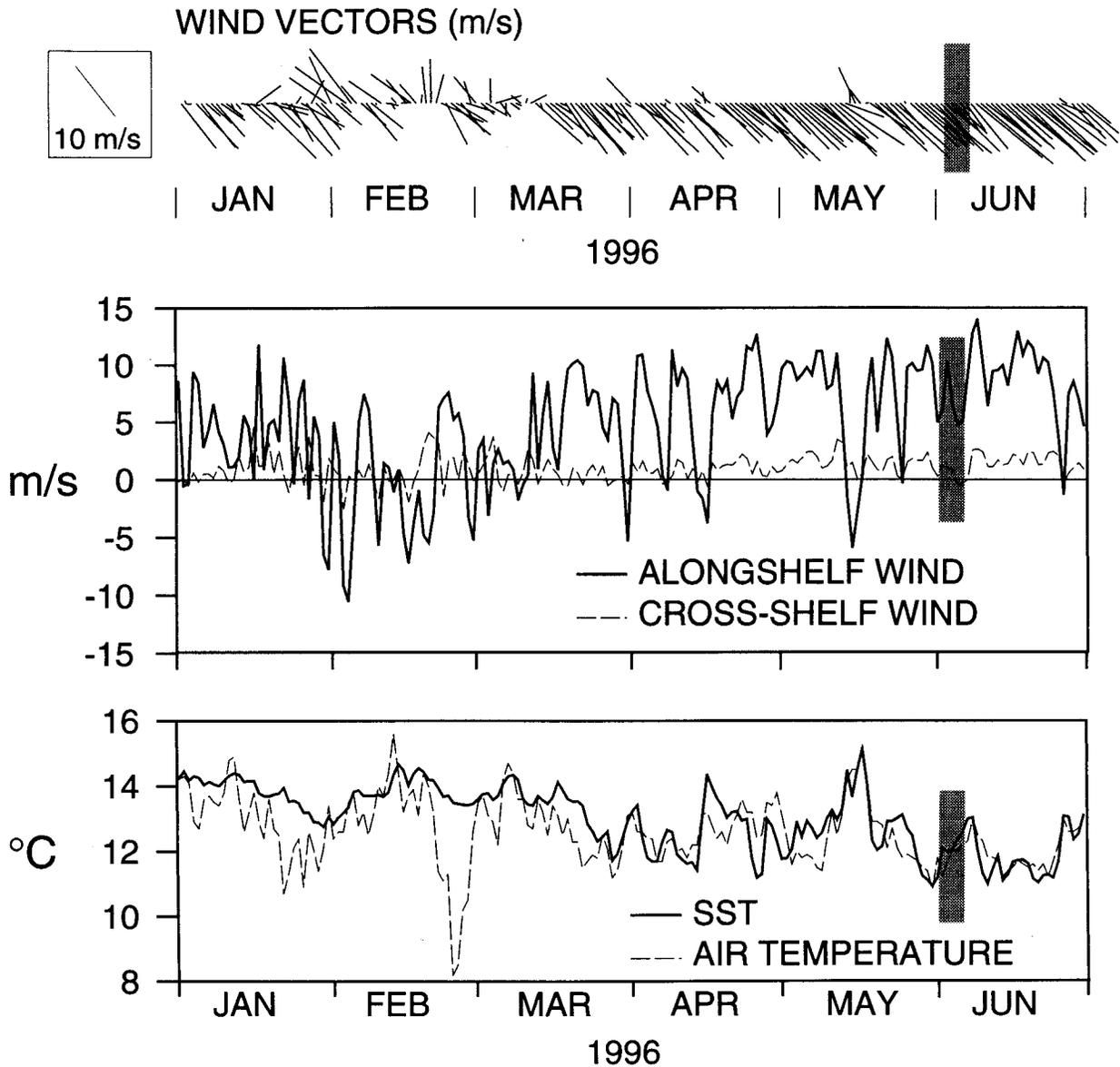
Figure 5a. Time series of meteorological and oceanographic data measured at NDBC buoy 46028 from 1 January to 30 June 1996. (Top) Daily average wind speed and direction (relative to true north); vectors point in direction that wind is blowing. (Center) Along-shelf (plotted as positive along 142°N orientation) and cross-shelf (plotted as positive along 52°N orientation) components of wind speed. (Bottom) Sea surface and air temperatures. The survey period is shaded.
