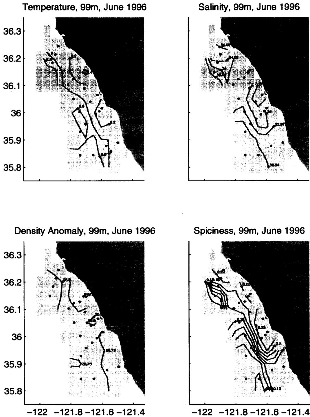
Figure 10. (a) Temperature, (b) salinity, (c) density anomaly, and (d) spiciness<sup>1</sup> measured at 99 m depth. Otherwise, same as Figure 9.
