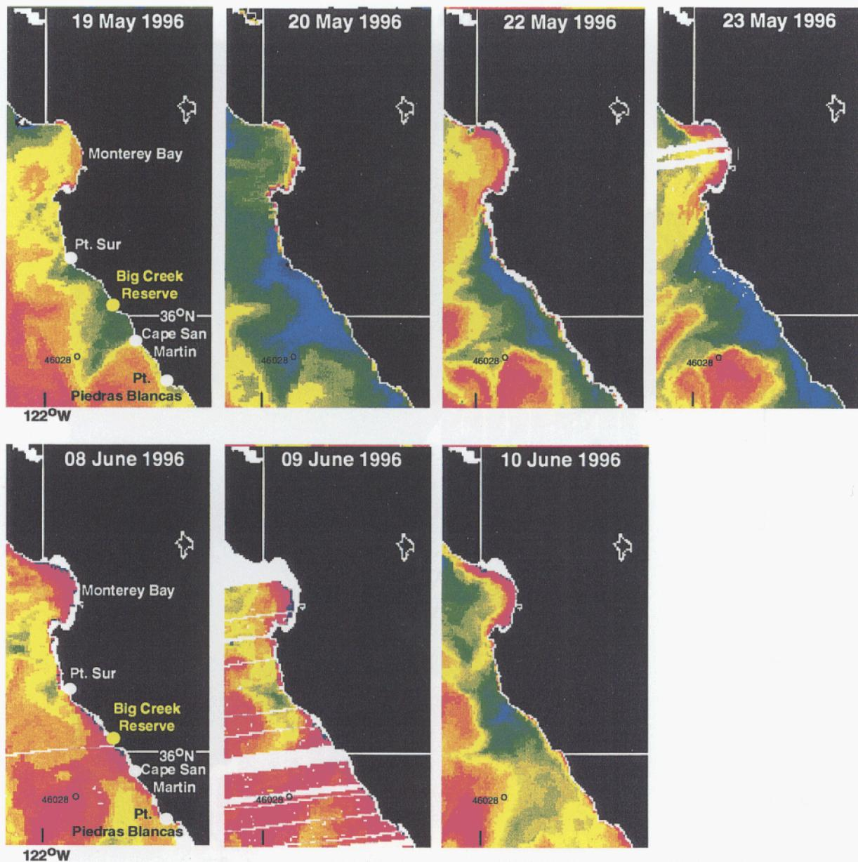
Figure 6. AVHRR satellite images of sea surface temperatures off central California from 19 May to 10 June 1996. A relative color scale is calibrated from coldest (dark blue) to warmest (fuchsia) temperatures. White stripes, especially evident in images on 23 May and 09 June, are due to data loss. Small open circle is location of NOAA NDBC buoy 46028.
