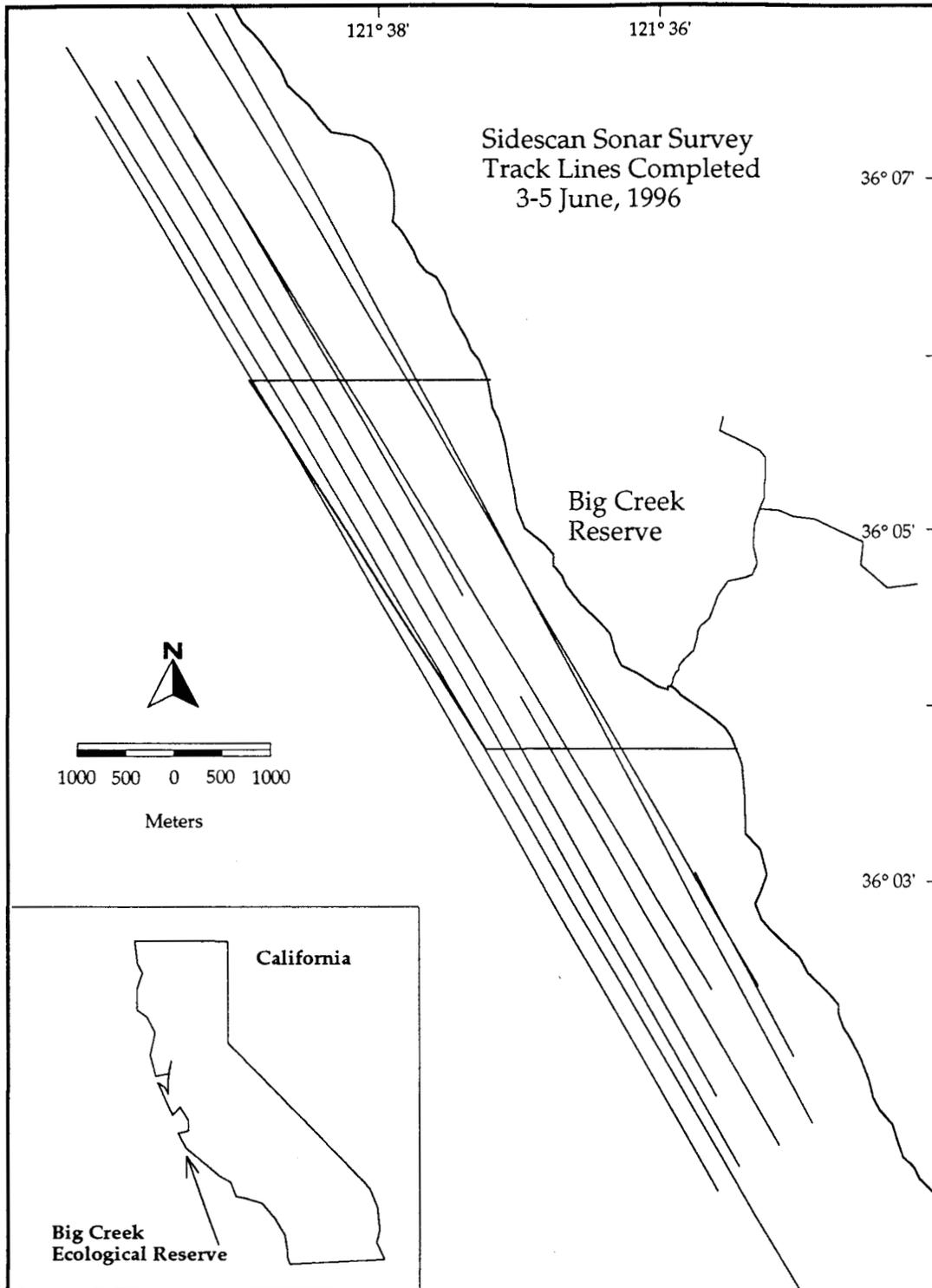
Figure 1. Location of the Big Creek Ecological Reserve and side scan sonar track lines completed during the geophysical survey of potential seafloor fish habitats on board NOAA ship *McArthur*.
