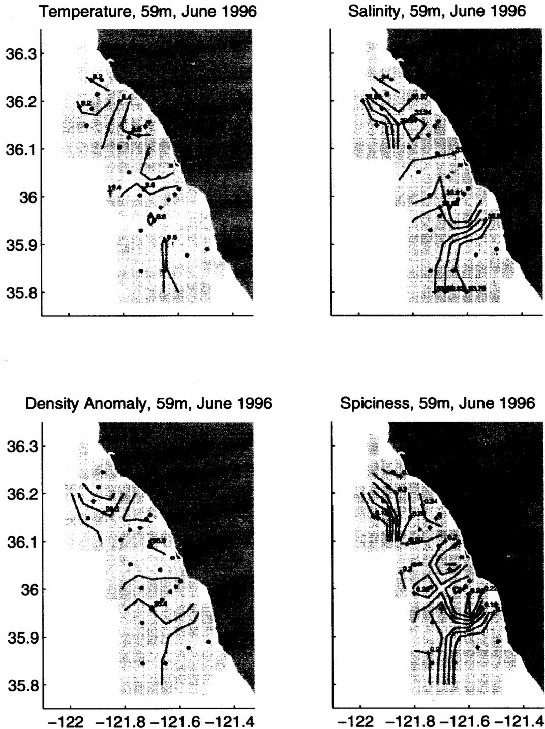
Figure 9. (a) Temperature, (b) salinity, (c) density anomaly, and (d) spiciness<sup>1</sup> measured at 59 m depth. Contour intervals are 0.2°C temperature, 0.03‰ salinity, 0.05 kg/m<sup>3</sup> density anomaly, and 0.02 spiciness. Otherwise, same as Figure 8.
