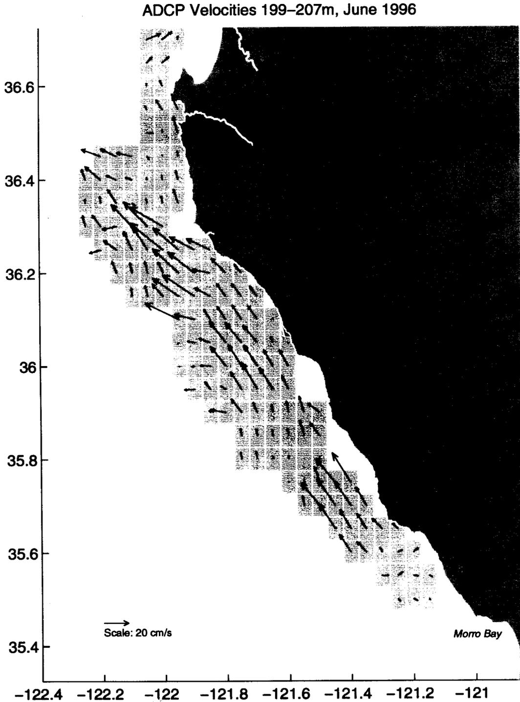
Figure 7d. Horizontal maps of ocean currents (ADCP velocity vectors) from Monterey to Morro Bays, 2-6 June 1996, averaged over 199-207 m water depth. Velocities over a (0.1 x 0.1)-degree region were gridded into 0.05-degree bins. Bins containing data are filled with light gray. The approximate region of the Big Creek Ecological Reserve is indicated with darker fill.
