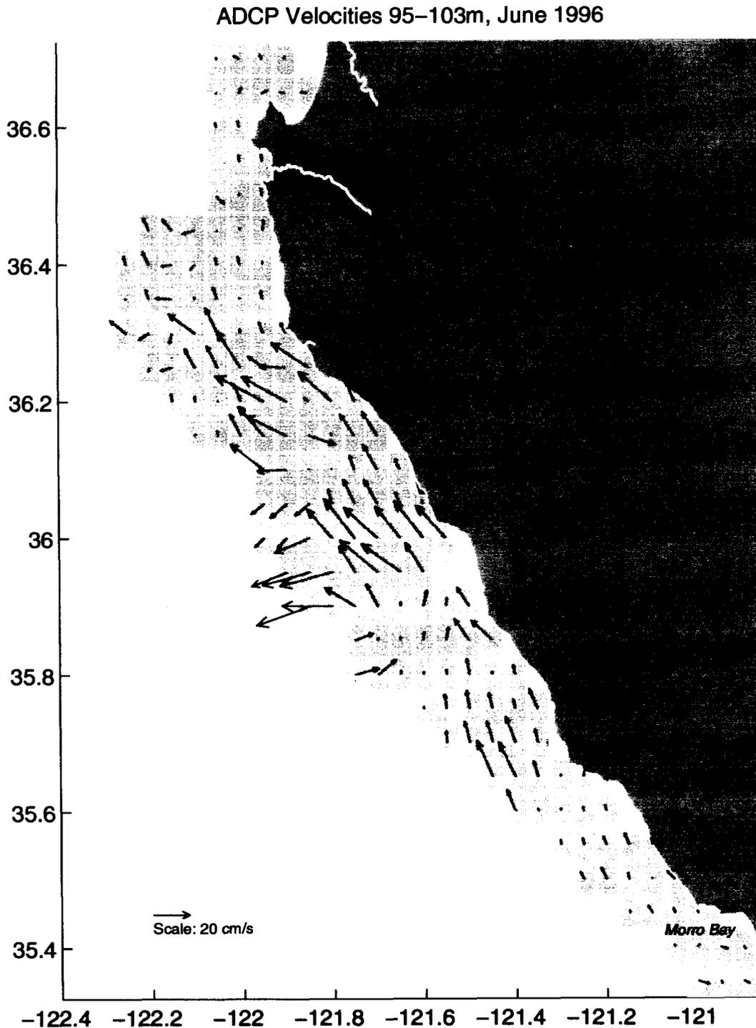
Figure 7c. Horizontal maps of ocean currents (ADCP velocity vectors) from Monterey to Morro Bays, 2-6 June 1996, averaged over 95-103 m water depth. Velocities over a (0.1 x 0.1)-degree region were gridded into 0.05-degree bins. Bins containing data are filled with light gray. The approximate region of the Big Creek Ecological Reserve is indicated with darker fill.
