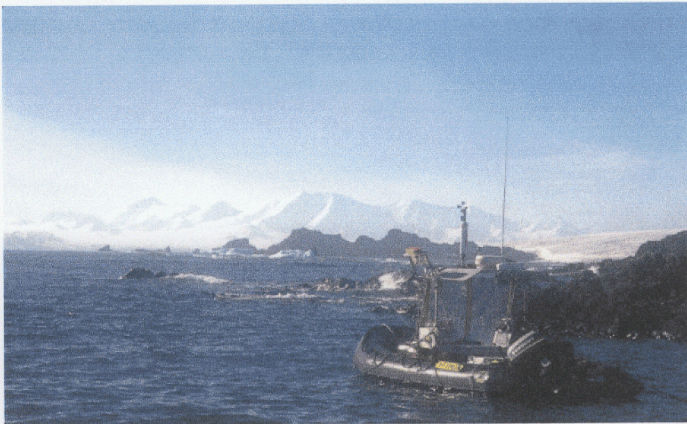
Figure 5.1 R/V Ernest four-point moored off Cape Shirreff, Livingston Island, Antarctica. The red 120kHz split-beam transducer sits atop the retracted arm (port-side); the WeatherPak 2000 meteorological station, radome, and 406MHz EPIRB are mounted on the cabin top; and the motorized down-rigger used for deploying the CTD and underwater video system is positioned near the steering station (starboard side).
