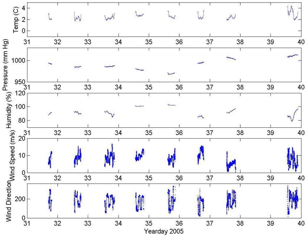
Figure 5.9 Meteorological data from R/V *Ernest* during the nearshore survey. The humidity sensor readings are likely offset 10-15% high. Mean wind speed was 8 m/s with a peak gust recorded of 17 m/s. Most frequent wind direction was from the SW and NW.
