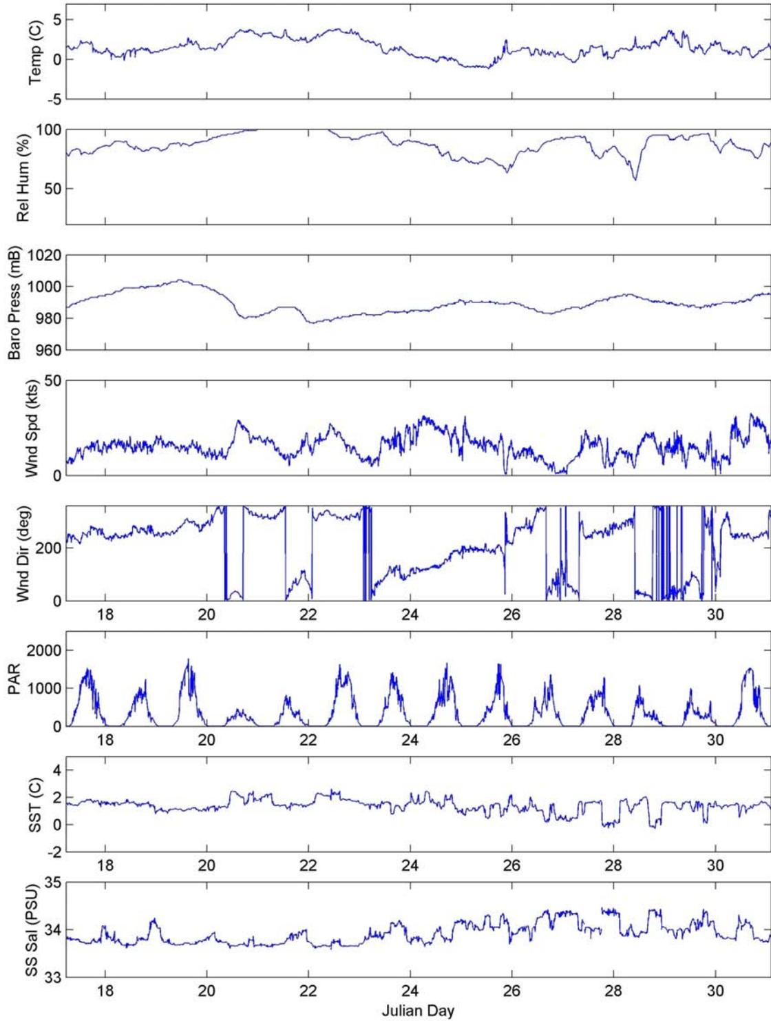
Figure 1.5 Meteorological data (5 minute averages) recorded between January 17<sup>th</sup> and January 31<sup>st</sup> during Leg I (survey only) of the AMLR 2004/05 Cruise. (PAR is photo-synthetically available radiation).
