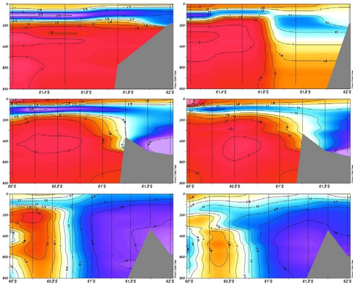
Figure 1.3 Vertical temperature profiles derived from CTD data recorded on three transects, W 05 (top), EI 03 (middle) & EI 07 (bottom), during Legs I (left column) & II (right column) of the AMLR 2004/05 South Shetland Island survey.
