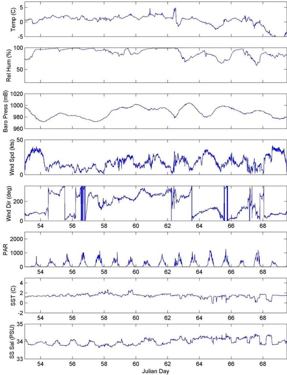
Figure 1.6. Meteorological data (5 minute averages) recorded between February 22<sup>nd</sup> and March 9<sup>th</sup> during Leg II (survey only) of the AMLR 2004/05 Cruise. (PAR is photo-synthetically available radiation).
