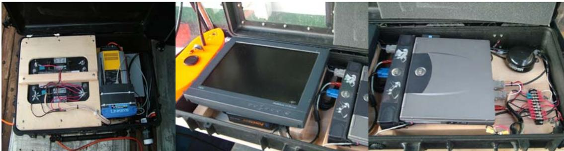
Figure 5.3 The two waterproof cases containing all of the equipment necessary to power (left), view (middle), collect and process (right) the acoustic, meteorologic, and hydrologic data from the RV *Ernest*.
