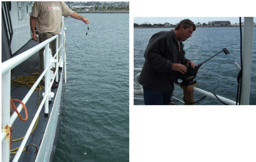
Figure. II.2. The calibration sphere and lead weight (left) suspended 2 m apart on monofilament line, and (right) one of the three remote-control downriggers used to position the target sphere.
