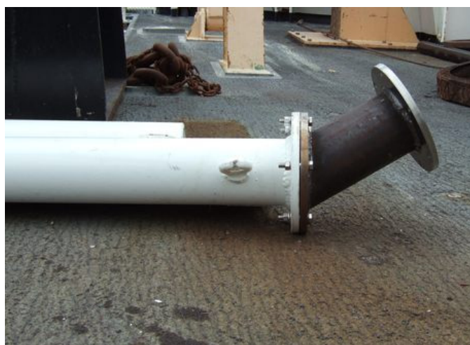
Figure II.25. Angled bracket for mounting the SM2000 head at 30° off-nadir to port on the bottom of the steel pole.
