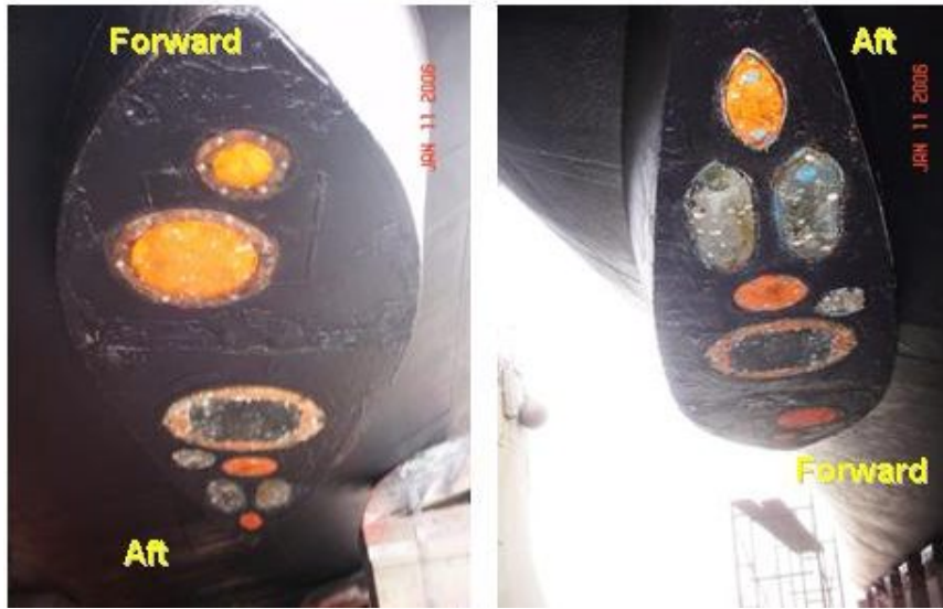
Figure II.3. Locations of the Simrad split-beam echosounder transducers on FRV David Starr Jordan .
