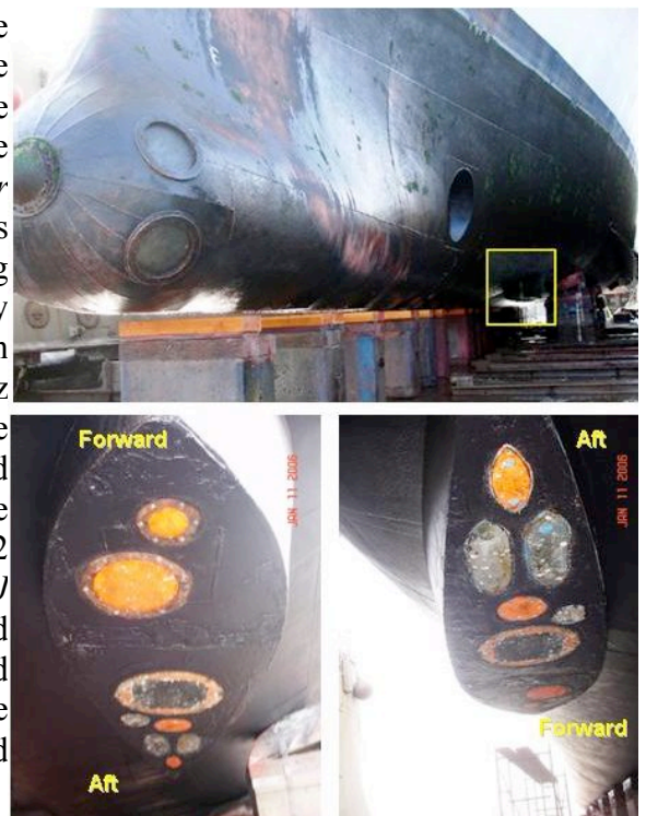
Figure 1. Locations and arrangement of EK60 transducers on David Starr Jordan .
