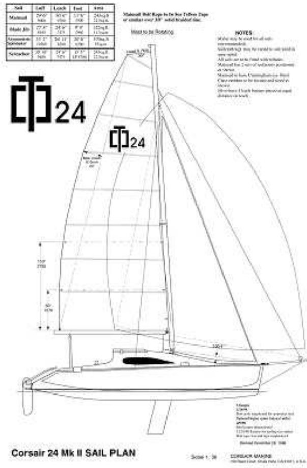
Figure 1. Corsair 24 specifications, sail plan, and accommodation layout.
