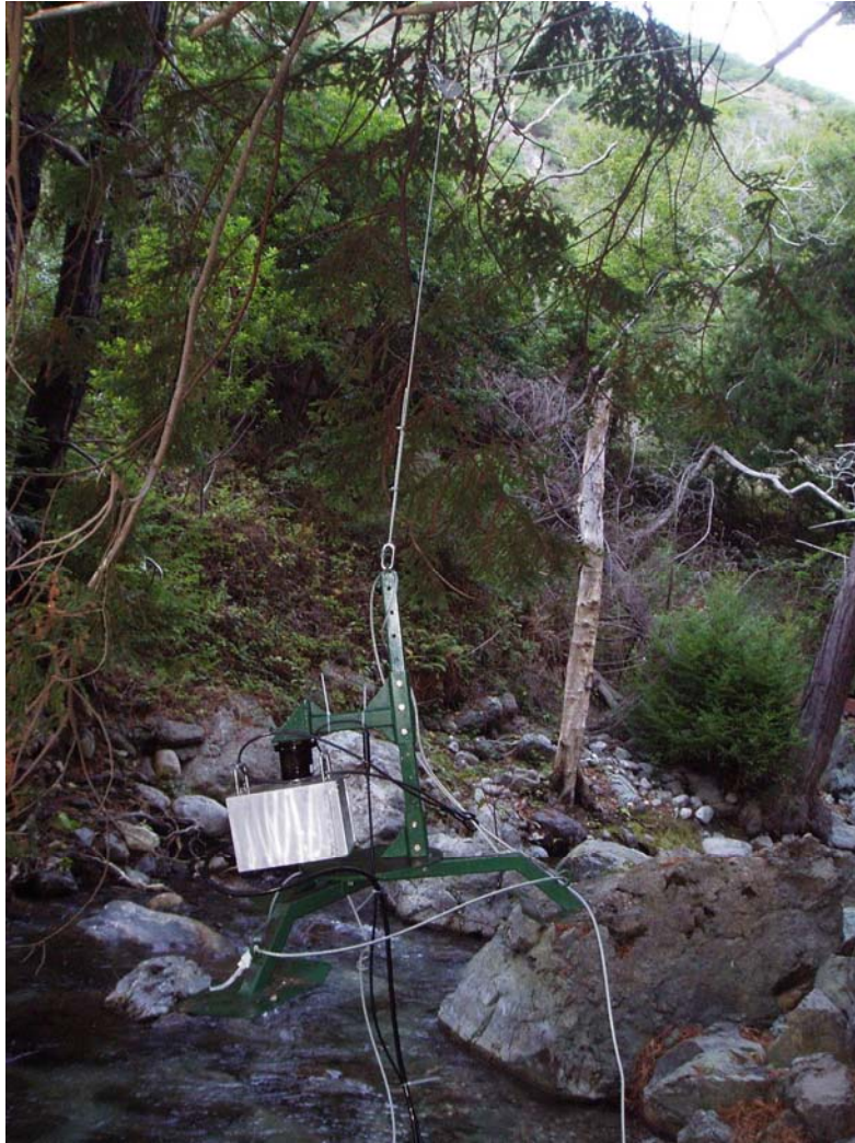
Figure 11. DIDSON hoist system supported by cabling across the stream at the Big Creek (Monterey County, CA) site.
