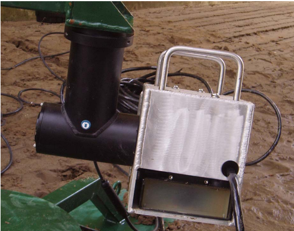
Figure 4. Pan and tilt rotator and aluminum housing around the DIDSON. The aluminum housing was designed to protect the DIDSON from debris floating downstream during high flow events. The dual axis pan and tilt rotator enabled remote sonar positioning.
