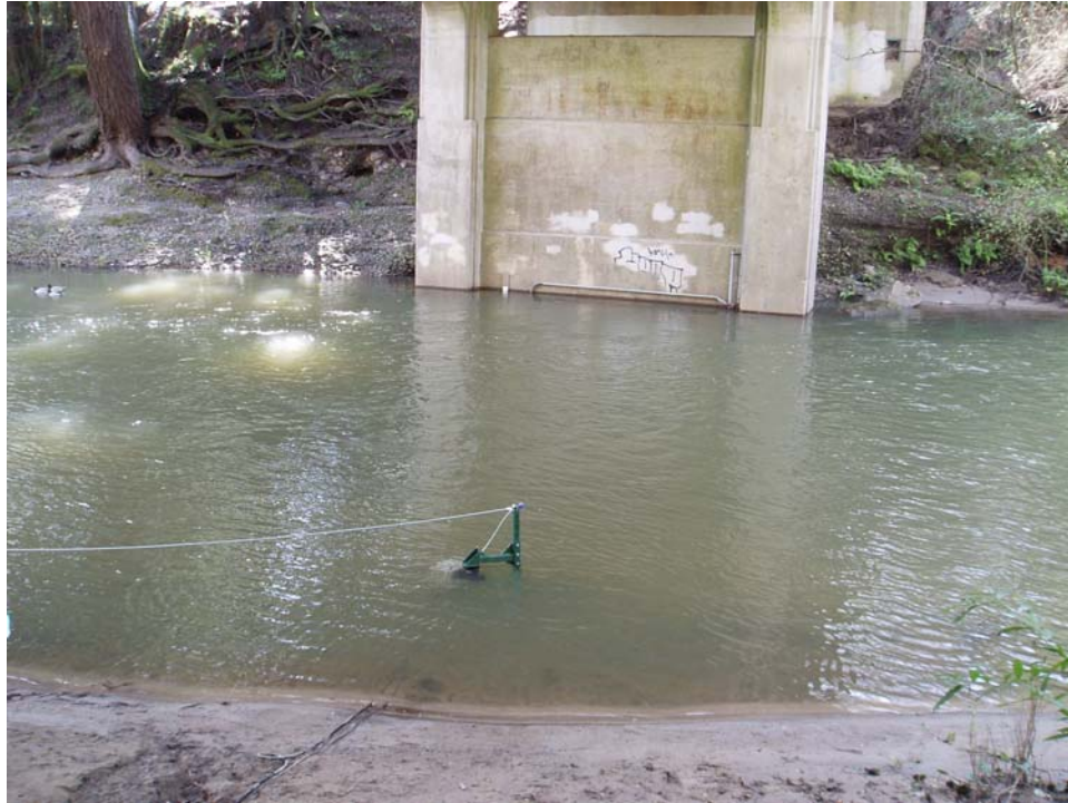
Figure 8. DIDSON study site on the San Lorenzo River (Santa Cruz County, CA). Note: this photograph was taken before deflector fencing was installed downstream of the sonar unit.
