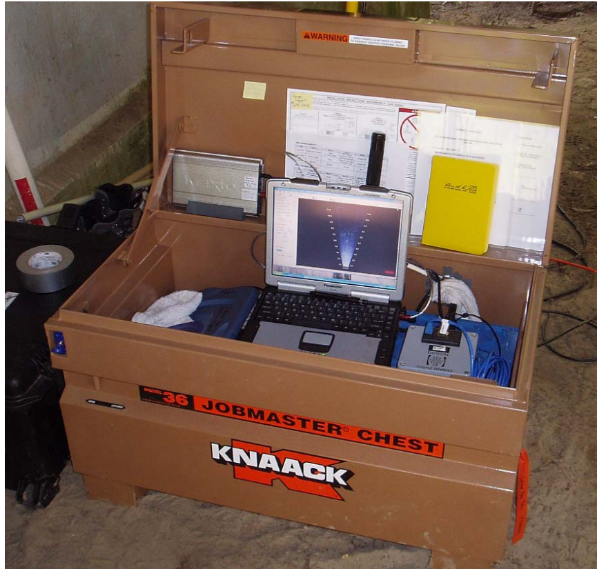
Figure 5. Weatherproof storage box for electronic components (i.e., laptop, external hard drive, back-up battery system, and DIDSON topside box). Box dimensions measured 56 cm high (closed position) x 48 cm wide x 91 cm long; 0.20 m 3 storage capacity; weight 44 kg.
