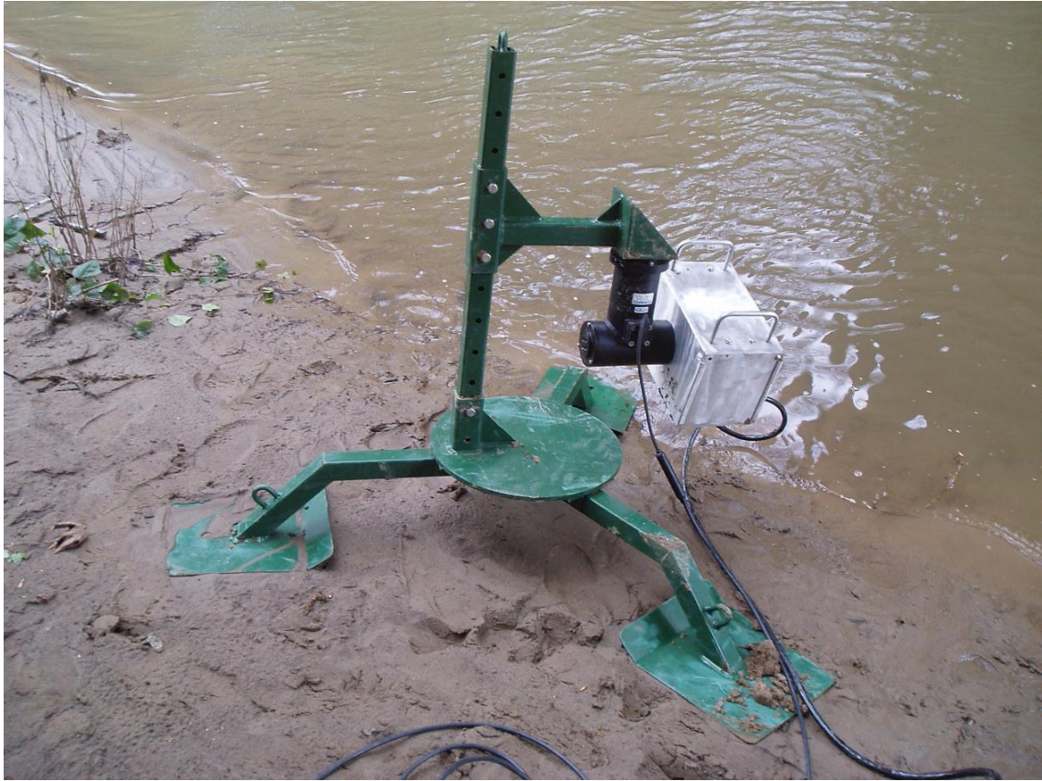
Figure 2. Tripod-style DIDSON mount showing adjustable ‘arm,’ sled-like ‘feet’ and sturdy base. This design was modeled after a mount used by the Alaska Department of Fish and Game.
