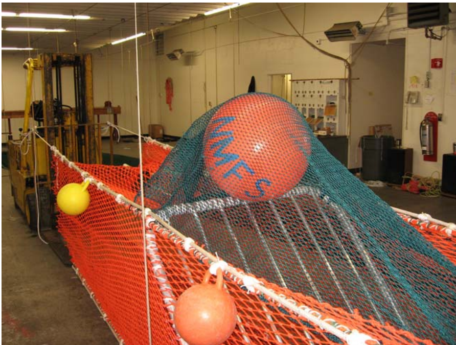
Figure 4. The MMED grate sewn into the intermediary panels with a large float demonstrating the escape panel above the grate.
