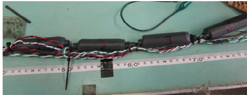
Figure 11. Pre-amp and depth sensors should be (a) attached to the steel cable using electrical ties and (b) together at the front end of the array assembly.
