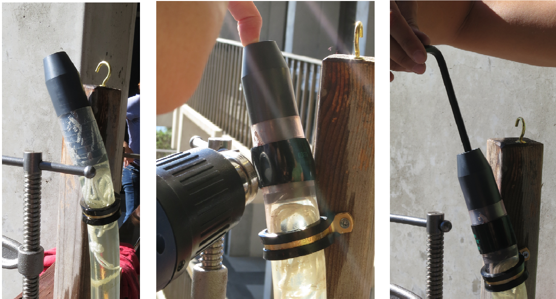
Figure 15. Once oil array is filled, end cap is put on the tubing, with a heat shrink hose clamp over the tubing at the position of the barbs. The screw is then placed in the end cap and tightened.
