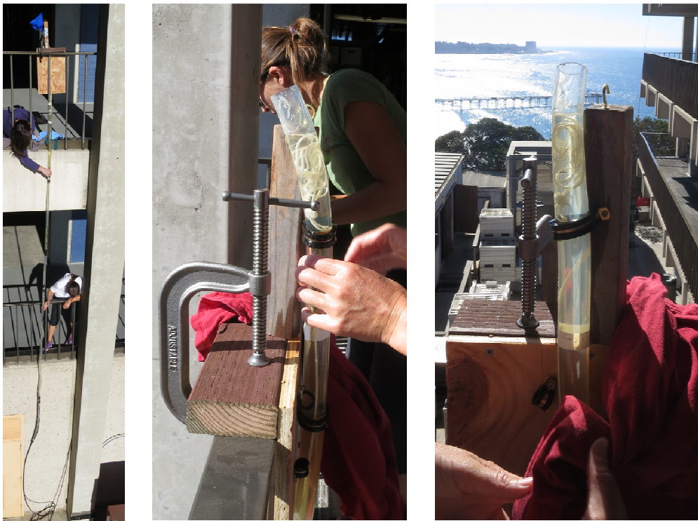
Figure 14. Array assembly should be hung vertically and filled with castor oil using a funnel.
