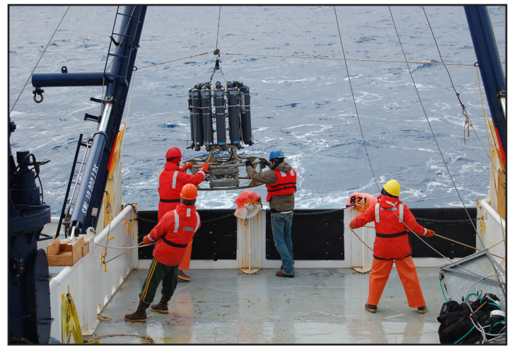
Deployment of the CTD from the R/V Moana Wave . Photo by Jen Walsh.
