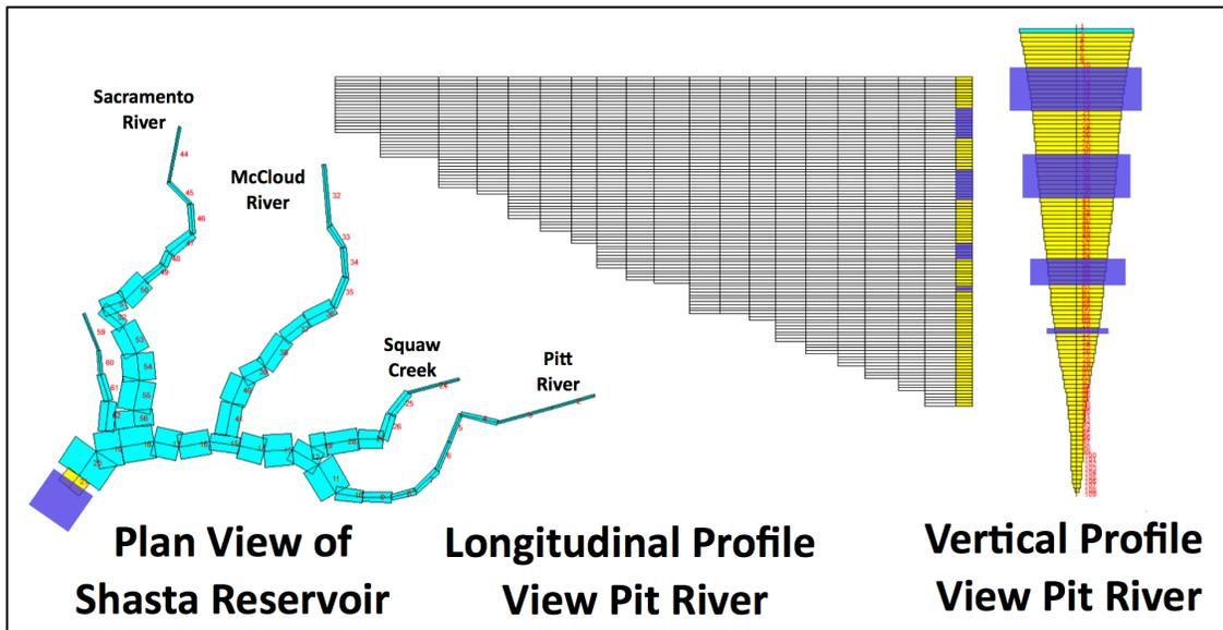
Figure 5: Geometry of the W2 model simulating water discharge and temperature in Shasta Reservoir, with location of the dam in plan view, and depths of the TCD gates in longitudinal (main branch of Pit River displayed) and vertical (at the downstream boundary of the dam) profile view denoted in purple. Note, the side gate does not technically have a width relative to other TCD gates and therefore a thin line is used to represent the elevation of the gate.
