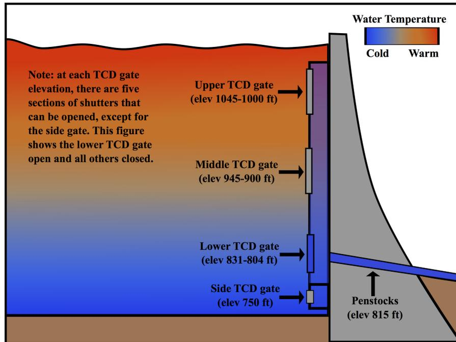
Figure 8: Conceptual schematic of the temperature control device (TCD) on Shasta Dam showing the locations and elevations of intake gates with elevations relative to mean sea level.
